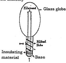
A light bulb is a relatively simple device consisting of a filament resting upon or somehow attached to two wires. The wires and the filament are conducting materials which allow charge to flow through them. Due to the joule effect, the filament produces light.
