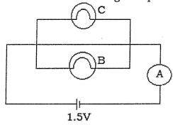
c) Calculate the electric current flow recorded by the ammeter A in the circuit if resistance of lamp C is 2 Ohms and that of lamp B is 3 Ohms.
